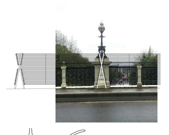
The proposal uses the lightest possible materials to make a highly flexible yet minimally obtrusive anti-climb barrier. It is normally striaght but when the weight of a climber is applied it would distort bending inwards and the cables lowering and closing up making hand holds difficult and increasing in bending as more weight is applied.
