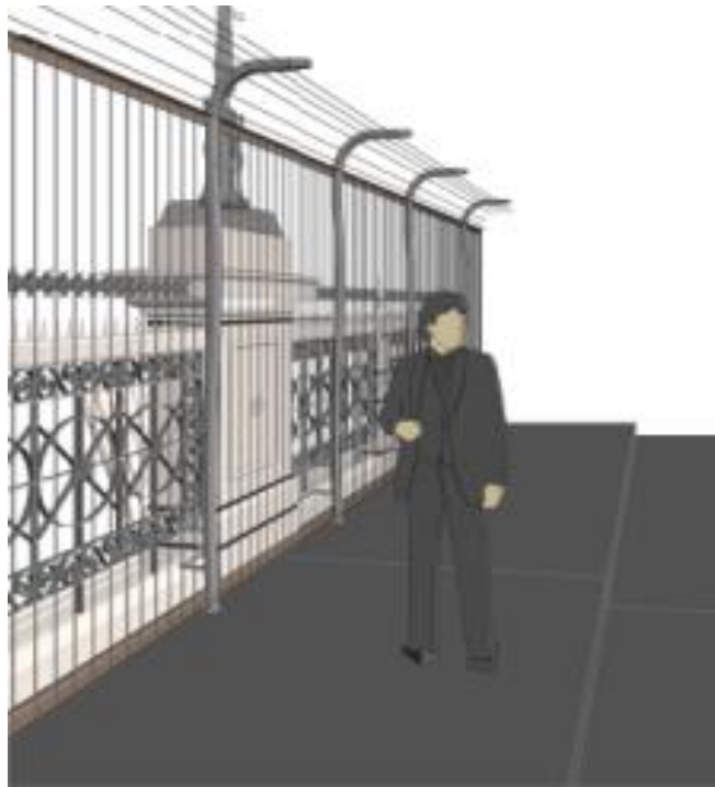
Schematic drawing showing the revised proposals, note visualisations overemphasize the vertical rods which will be only 8mm thick
